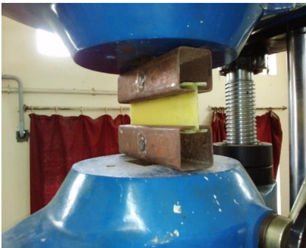
Fig- 6: 1 st I-Beam Specimen with Araldite 2015 Adhesive Before Test
