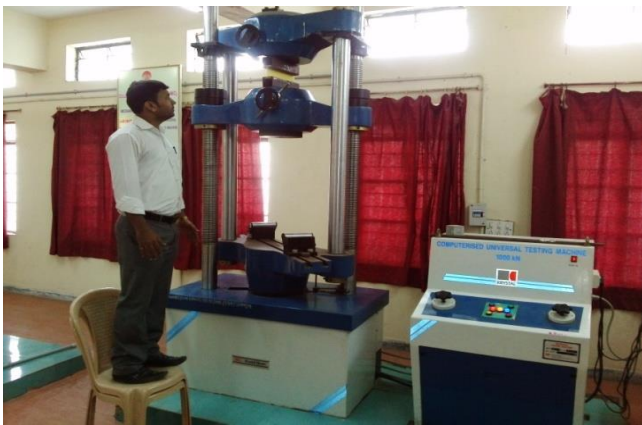
Fig- 5: Experimental Setup of Composite I-Beam Tensile Testing
