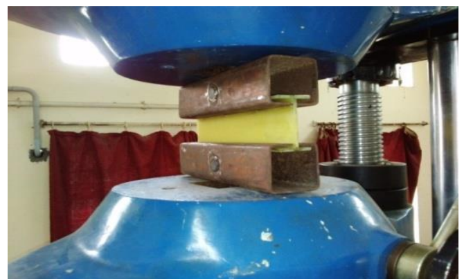
Fig- 7: 2 nd I-Beam with Hundsman Araldite Adhesive Before Tensile Test
