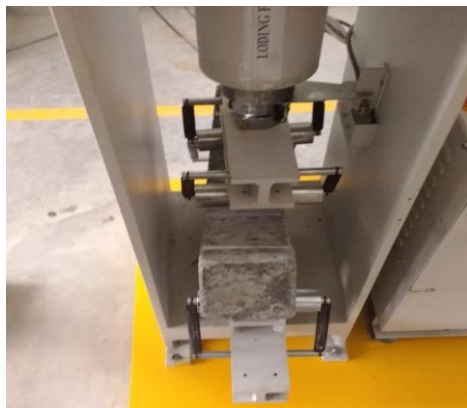
Figure 6: Cylinder under Flexural Testing Machine
