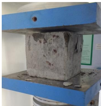
Figure 4: Cube under Compression Testing Machine
