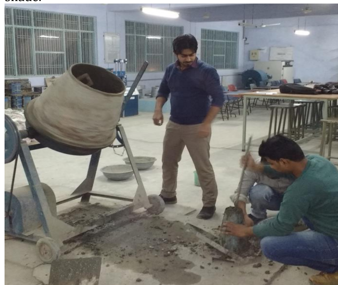
Figure 3: Workability Test using Slump Cone Table - 1: Concrete Mix with Different Proportion
