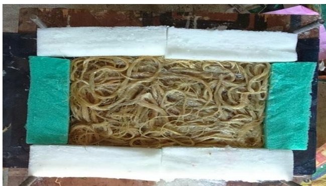
FIG 3.1 : Mixture Of Fiber And Resin Applied On The Wooden Pattern Board
