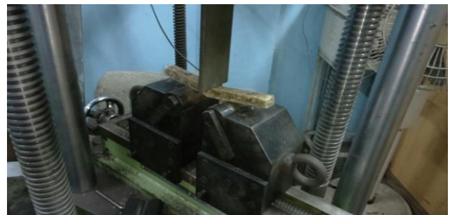
Fig 3.4 Broken Specimen After the load is applied in Universal Testing machine
