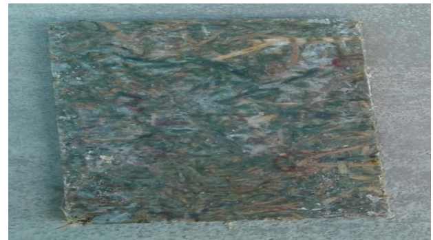
FIG 3.2 Banana Fibre Composites Brought Out From The Wooden Board
