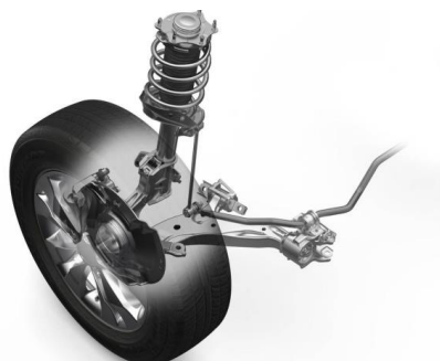
Fig-2: McPherson Strut (A type of Independent suspensions)
