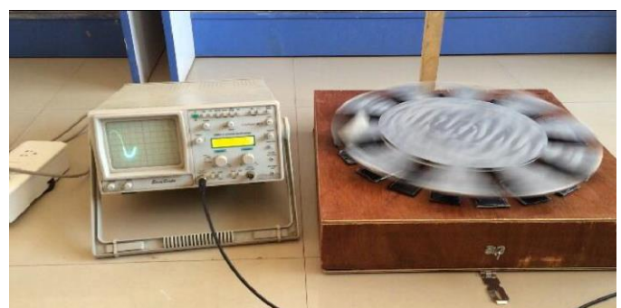
Fig-5: Testing of prototype output on C.R.O
