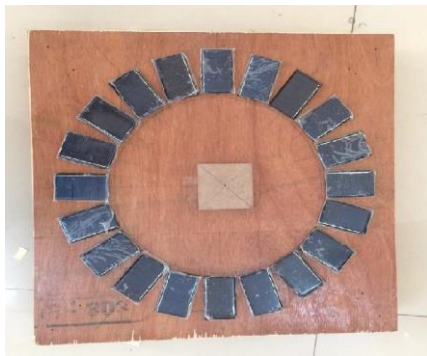
Fig -2: Construction of Base for components mounting
