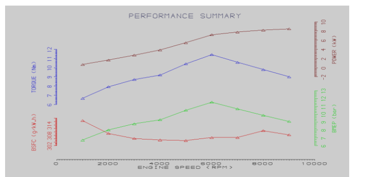
Fig-6: Graph for intake length 385.07mm(6000rpm)
