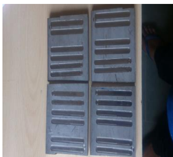
Fig-4 Work-piece material Alloy steel 316I
