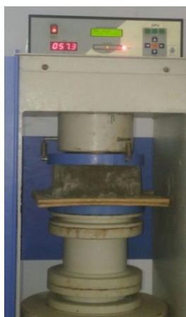
Fig -5: Compressive strength test on foam concrete brick
