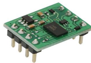
Fig -10: Vibration sensor
