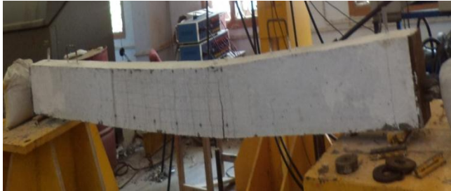
Fig.22. Crack Pattern of GPC Post Tensioned Beam
