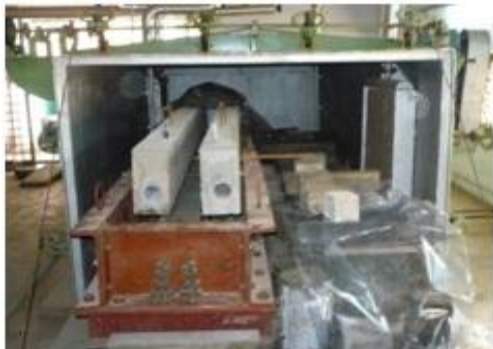
Fig.18. Specimens inside Steam Curing Chamber
