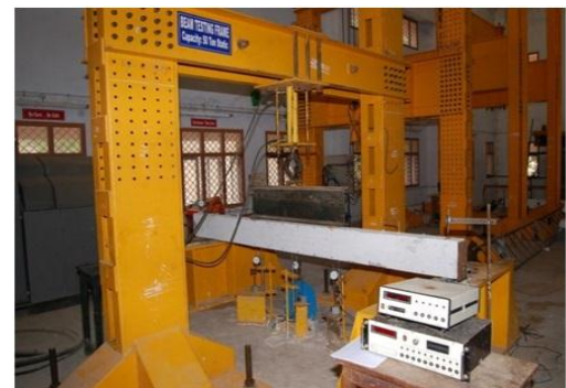
Fig.20. Experimental Setup of Beam
