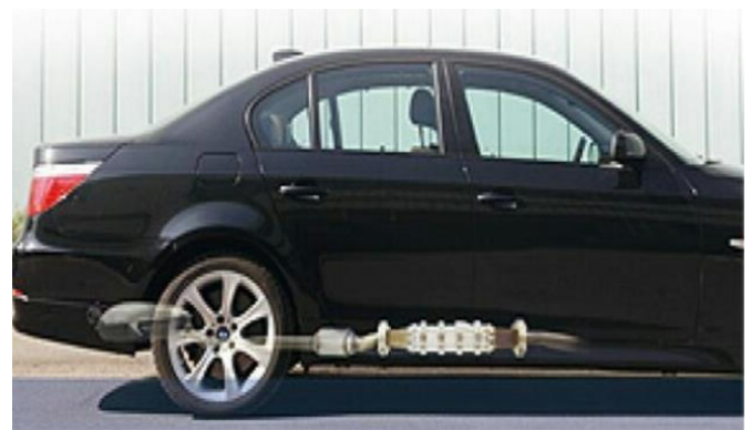
Fig.3 BMW prototype vehicle using TEG waste heat recovery
