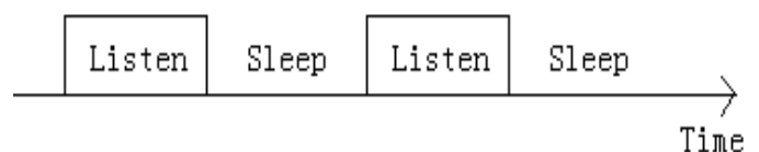
Figure-1 Frame= T_{listen} + T_{sleep}
