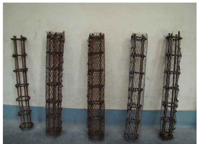
Fig 3: Reinforcement of specimen details
