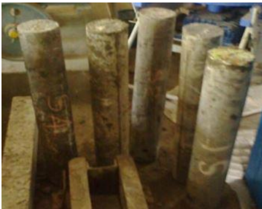
Fig 5: Column specimens after curing
