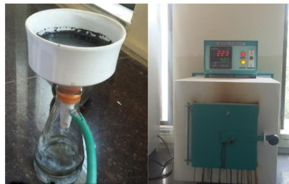
Fig-3 (A): Natural filtration process for carbon content Fig-3 (B): Incineration of rice husk
