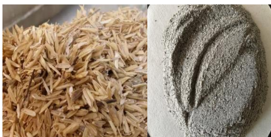
Fig-2 (A): Natural rice husk. Fig-2 (B): Natural rice husk after burning.
