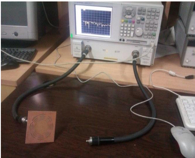
Fig 15: Return Loss characteristics of designed antenna at VNA screen.
