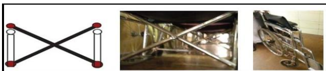
Figure 3. Cross brace bar mechanism
