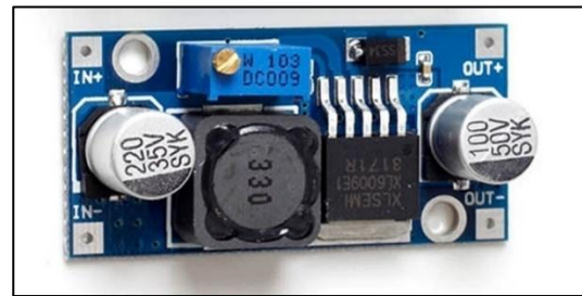
Fig-4: Buck-Boost converter
