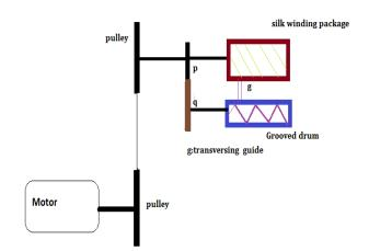
Fig.5 Precision winding principle
