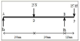
Fig 4.3.2 Vertical loading diagram
