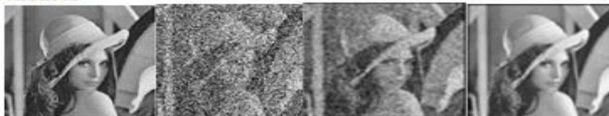
Figure 8 De-noising performances of Translation Invariance Algorithm for wavelets filter under various noise conditions. (a) Original Image (b) Noised Image (c) Without TI De-noised image (d) With TI De-noised image.
