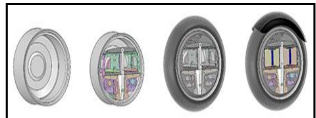
Fig-9: Hidden Motors and Drive
