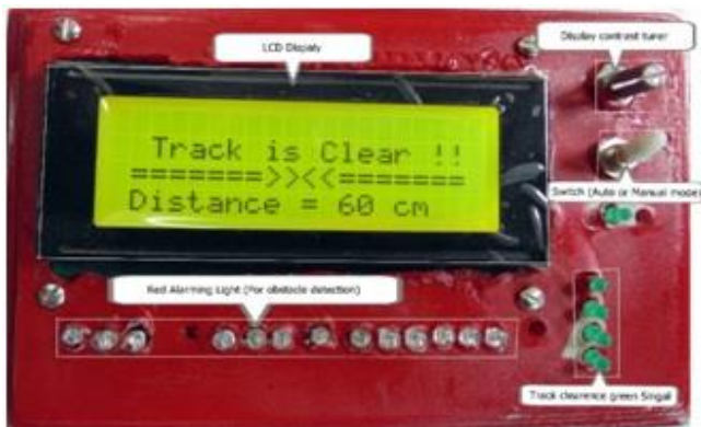
Fig-5: Our designed control device (Front side).
