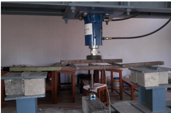
Fig -5: Testing of channel section
