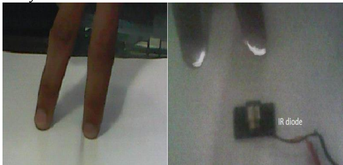
Fig. Fingers cutting the infra red beam close to surface Fig. Infra red visible through camera( filter is used )
