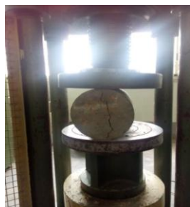
Fig 6: split tensile strength test
