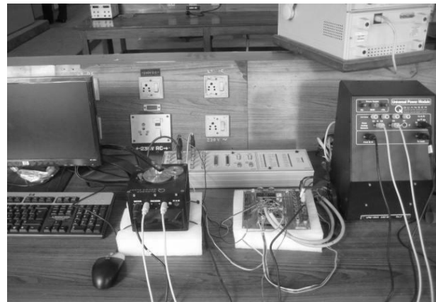
Fig-2: Experimental set up of SRV02
