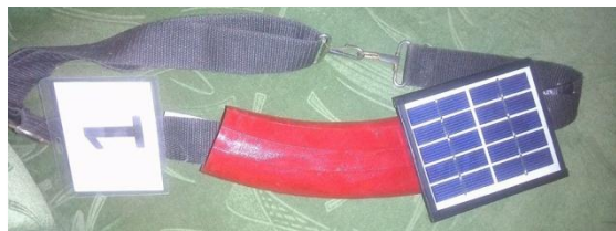
Figure 7B: collar circuit covered
