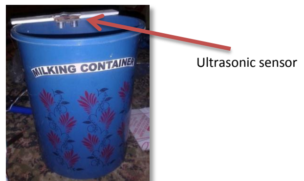
Figure 10: Milk volume measurement container
