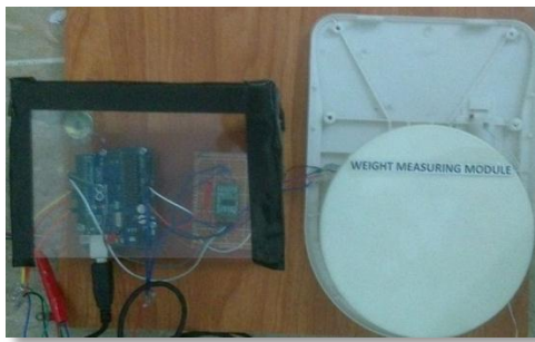
Figure 11: weight measuring circuit
