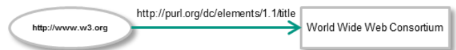
Figure 4: Example of an RDF Graph with subject, predicate and object and representation in XML.
