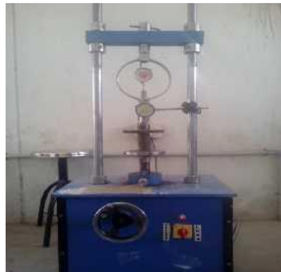
Fig-2: Unconfined Compressive Strength Test
