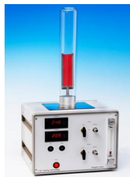
Fig 2. Experimental Set Up Of LOI Test
