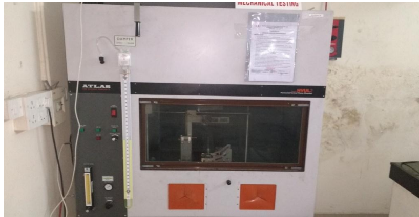
Fig 3. Horizontal and vertical test chamber gas torch
