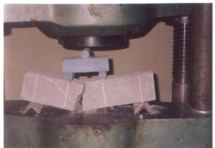
Fig:10 TYPICAL FRACTURE PATTERN OF BEAM SPECIMENS DUE TO FLEXURAL LOAD ( M30, 0% Fly ash)
