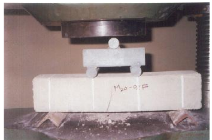
Fig: 9 TYPICAL FRACTURE PATTERN OF BEAM SPECIMENS DUE TO FLEXURAL LOAD (M20, 0% Flyash)
