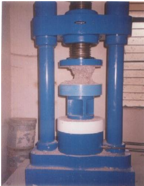
Fig: 8 TYPICAL FRACTURE PATTERN OF CUBE SPECIMENS DUE TO COMPRESSION LOAD
