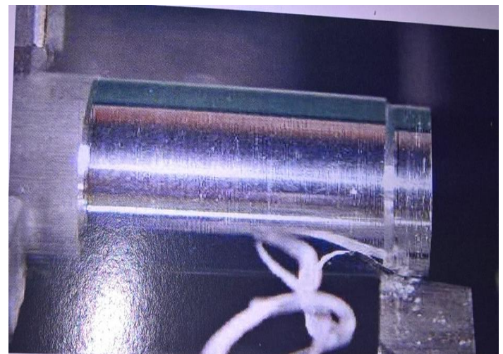
Fig.5. 99.4%Aluminium material turning
