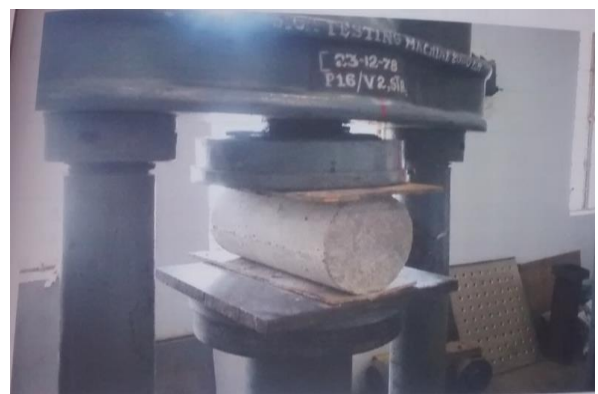
Fig -2: Split tensile Strength – Experimental set up
