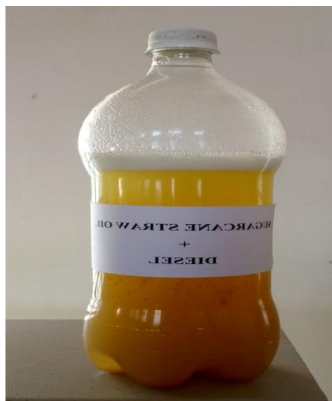
Fig 3: Sugarcane Straw Bio – oil blended with Diesel
