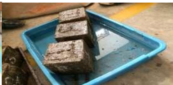
Fig 3: Sorptivity test setup of concrete blocks
