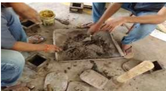
Fig 1: Mixing process of concrete
