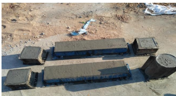
Fig-3 : Specimen Casting after proper compaction
