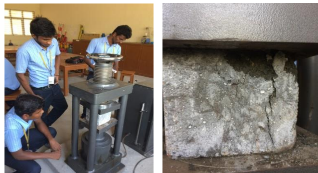
Fig -4 : Compressive strength setup
