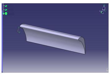
9. This base which is in shape of I-section is Extruded by using PAD DEFINTION
