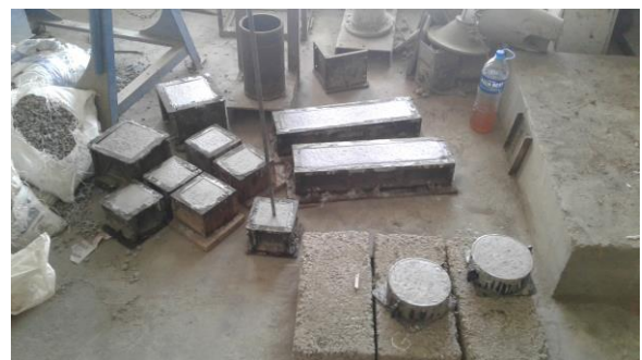
Figure - 3.0 Casting of HSC Cylinders.
