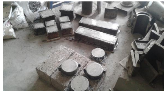
Figure - 2.0 Specimens prepared for casting.
