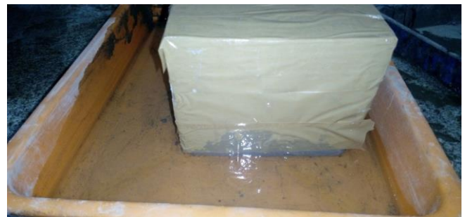
Figure - 7.0 Schematic of Sorptivity Test.
