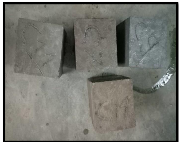
Fig -4: Cubes after curing
