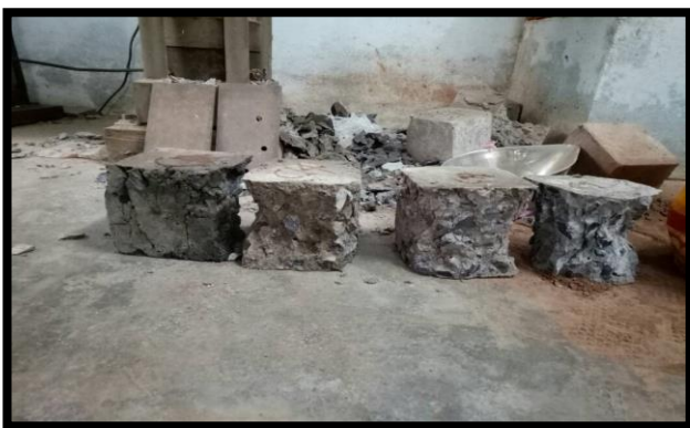
Fig -6: Cubes specimen after testing
