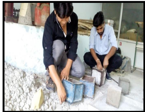
Fig -3: Demoulding of cubes
