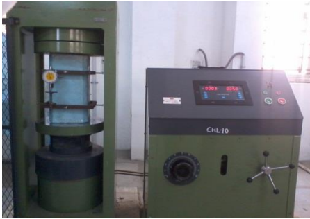
Fig - 3. Specimen in compression testing machine
