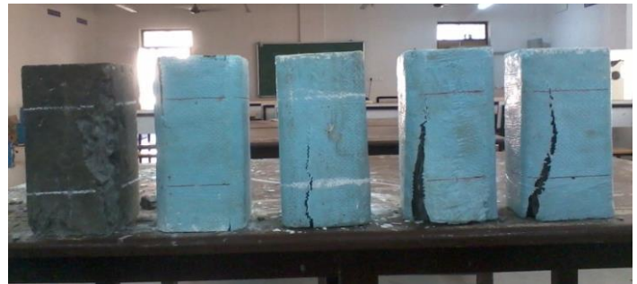
Fig - 5. Failure crack of concrete prisms
