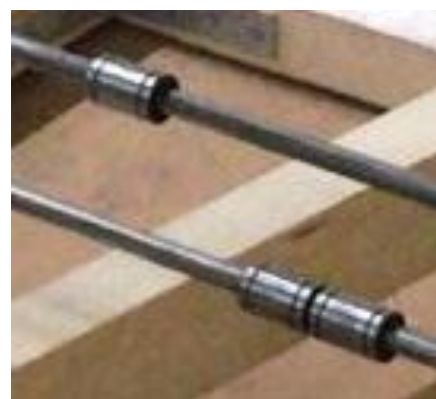
Fig 5: Linear slide bearings on guide rail
