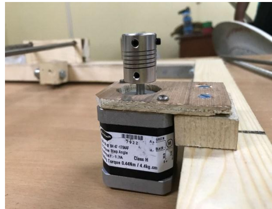
Fig 8: Stepper motor coupling mounted over motor
