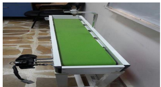
Fig-11: DC motor connection to the conveyor system.
