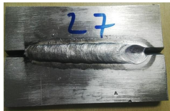
Fig-2: Work piece after welding
