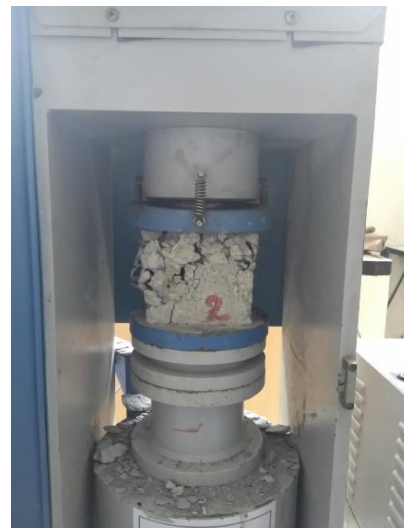
Figure 2 Cube test of Pervious concrete
