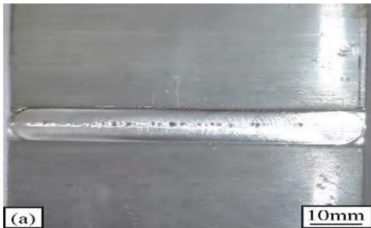
Fig-4(a):Top view of weld (800mm/min)
