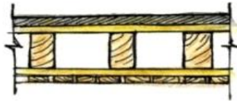
Fig -16: Traditional wooden ceilings expand during flood & contract afterwards causing walls to crack (Source: Author)
