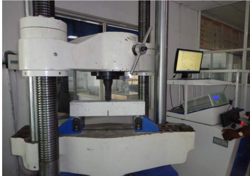
Fig 3: Servo Controlled UTM for Fracture Test
