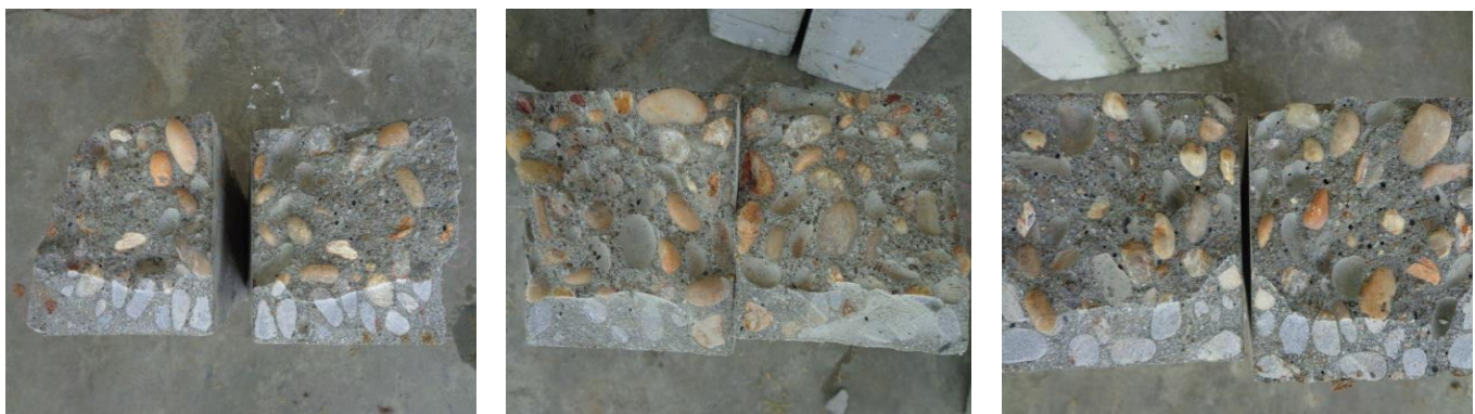
a) (b) (c) Fig 14: Fractured surfaces of River Gravel Concrete for: (a) M 30; (b) M 50; and (c) M 70
