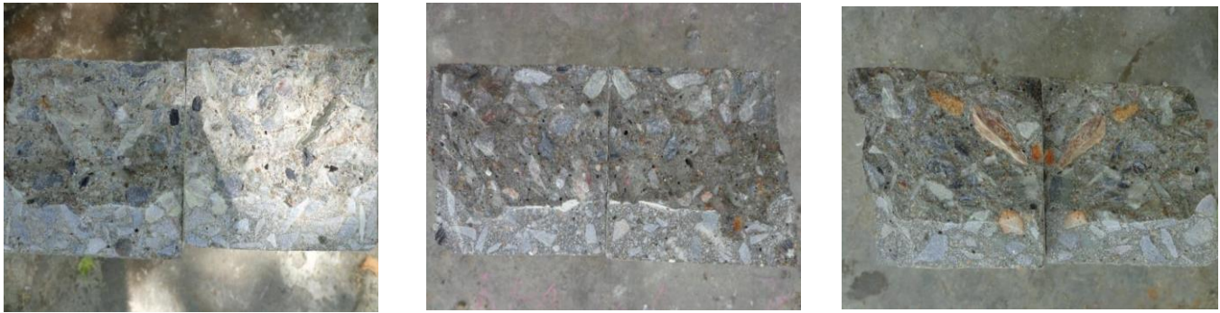
(a) (b) (c) Fig 13: Fractured surfaces of Quartzite Concrete for: (a) M 30; (b) M 50; and (c) M 70
