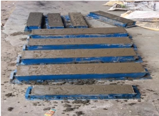
Figure 3 Casting of Beam
