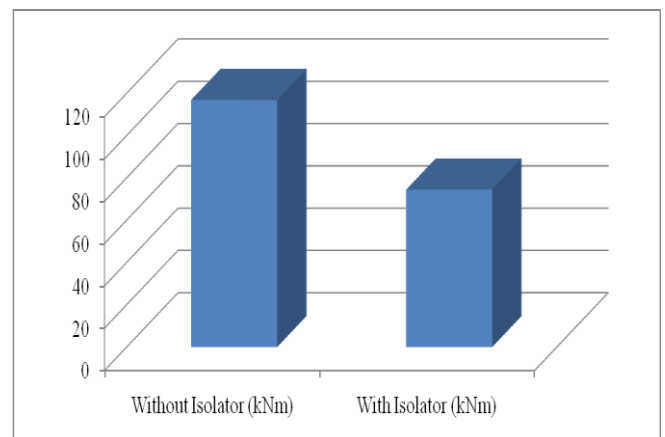
Chart -7: Maximum Shear Force in Columns at Bottom Storey for Both with and Without Isolator Building (Symmetrical)
