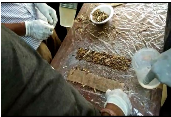
Fig 2.4: Hand lay-up Process
