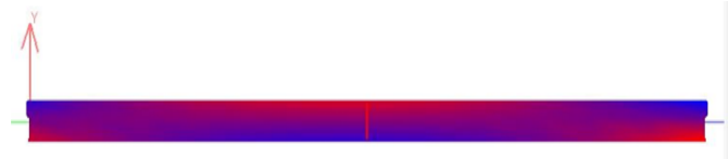
Fig -3: Stress in Composite Beam Longitudinal Section
